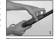
4. Keeping the hinge pin notch engaged with the hinge pin, lift the nose of the barrels until the action closes. Caution: If you attempt to close the gun and the barrels bind or don't seem to fit then the hinge pin and notch are not engaged. DO NOT FORCE, try again. Release the hinge pin and notch and the barrels will be locked in place.
